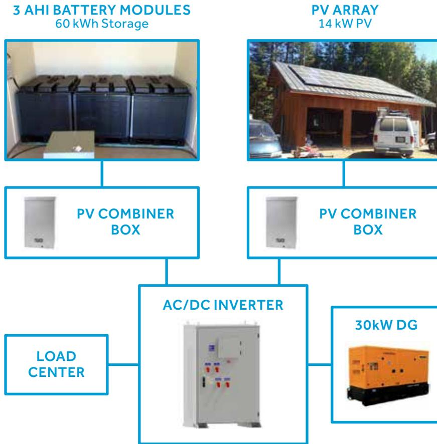
Figure 10: Block diagram of Redwood Gate Ranch microgrid
